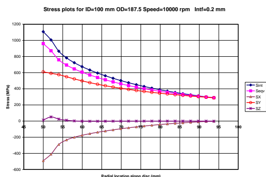
Fig 4.13 Graph showing variation Stresses in radial direction for Outer diameter 187.5 mm.
