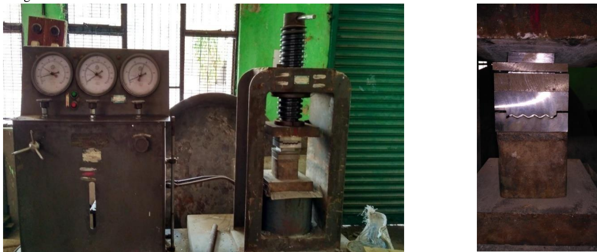
Fig.4: a) Hydraulic Press (b) specimen sandwich between the corrugated die and flat die
