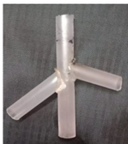
Fig.4: 3D Printed Phantom (blood vessel)
