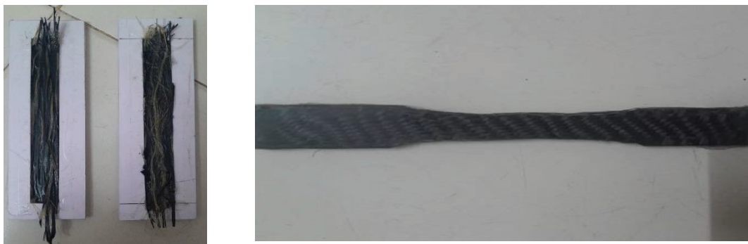
Fig 2: Preparation of Specimen as per the standard of ASTM D638-14
