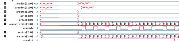
Fig. 5-3. Read Address Channel Results - The waveform shows that there is correct read request acceptance and burst parameter decoding.
