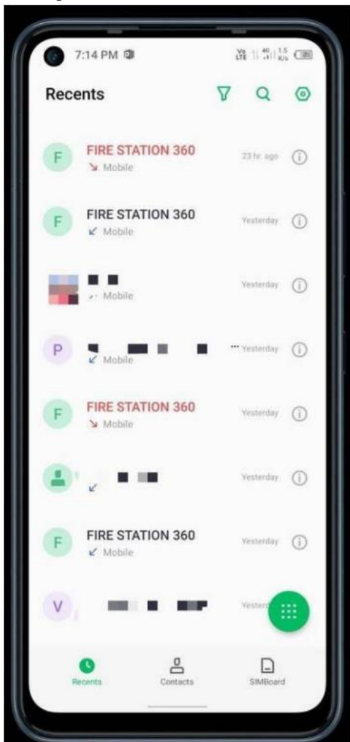
Fig. 7. shows a phone call log. This log contains information about outgoing and incoming calls of the Fire Station 360 GSM module as part of the test. The contacts will be under the system name, which is FIRE STATION 360. This has proven that the SIM900A module was able to connect to the cellular network and manage call dispatch.
