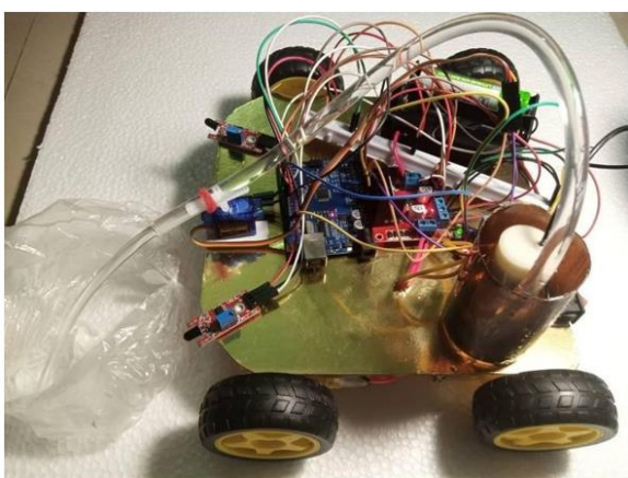
Fig. 6. Firefighting robot - rear/quarter view, and there is the 18650 lithium-ion battery pack, four BO gear motors with rubber tires, and the water reservoir. The acrylic tube that runs out of the tank cap and the nozzle servo assembly which is on the front side of the platform is clearly and obviously attached.
