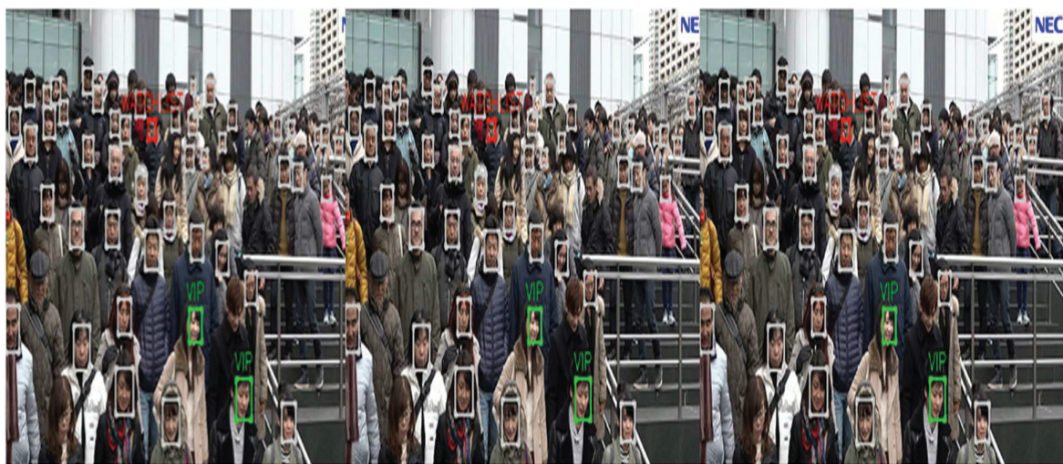
Fig. 6: (a) Result detected by Face SSD, (b) Face Detected by MTCNN, (c) Face Detected by YOLO- Face
