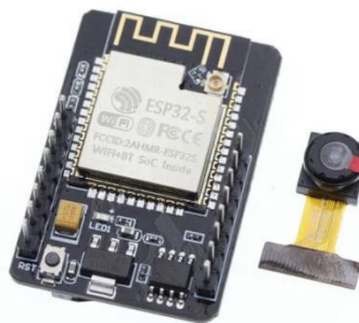
Figure 3. ESP32 CAM WiFi Module Bluetooth with OV2640/RHYX-M21-45 Camera
