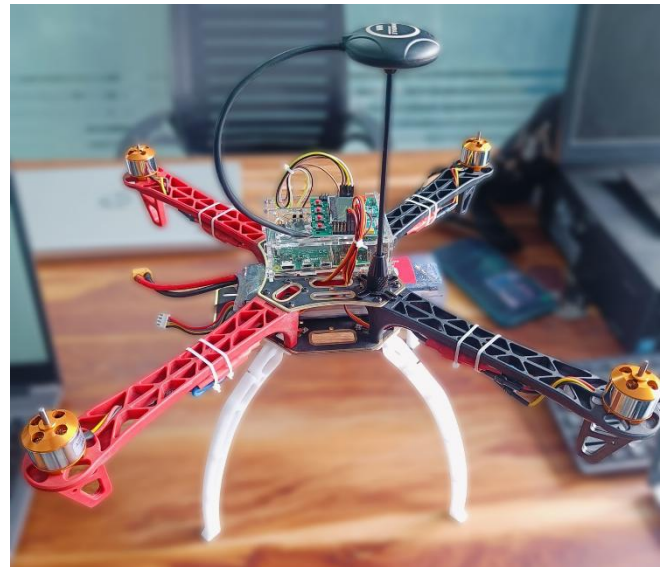
Figure 3: Assembled gesture-controlled drone used for system implementation (Image shows GPS module, propellers, and wiring setup as described above.)
