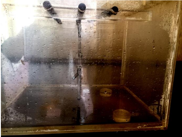
Shows the component loaded inside the salt spray chamber in hangers.
