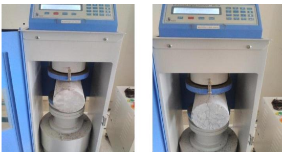
Split tensile testing on cylinder
