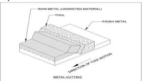
Cutting processes work by causing fracture of the material that is processed. Usually, the portion that is fractured away is in small sized pieces, called chips. Common cutting processes include sawing, shaping (or planning), broaching, drilling, grinding, turning and milling. Although the actual machines, tools and processes for cutting look very different from each other, the basic mechanism for causing the fracture can be understood by just a simple model called for orthogonal cutting.
