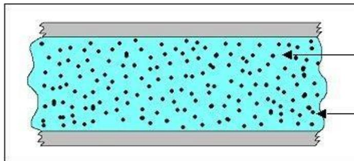
When a magnetic field is applied, however, the microscopic particles (usually in the 0.1–10 μm range) align themselves along the lines of magnetic flux, see below.
