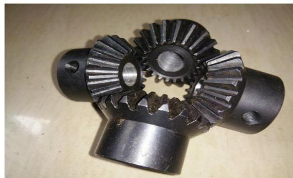
**Fig.3 Bevel gear**
