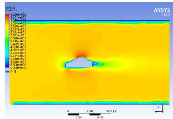
**Result for when Diffuser section at 11 Degree:**
