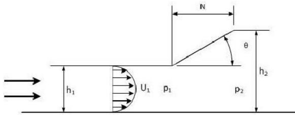
Figure 1. Shows velocity profile of diffuser.
