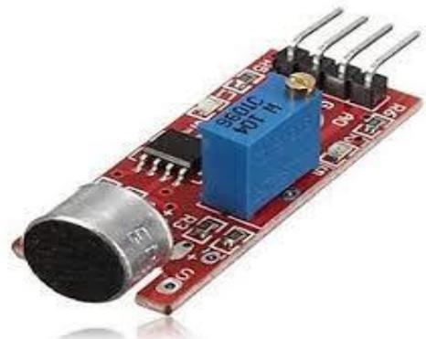
Fig -5: Acoustic Sensor
