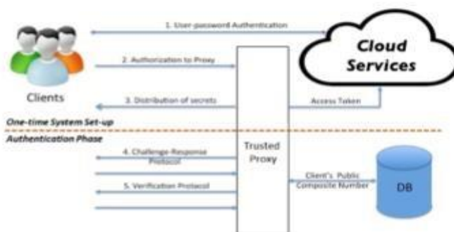
Fig. 1. System Architecture of the cloud-based authentication protocol
