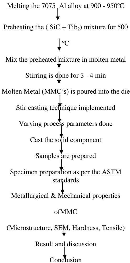
STIR CASTING ROUTE FOR FABRICATION OF MMC:
