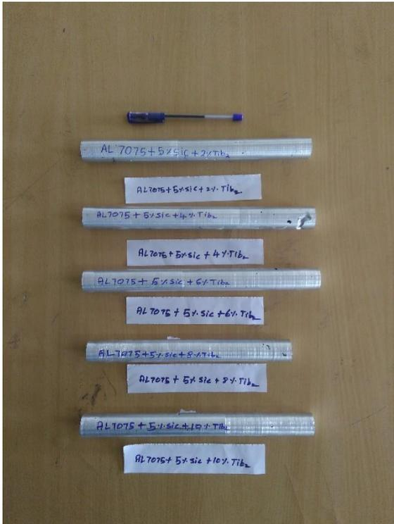
Figure: Stir casting Metal Matrix Composition
