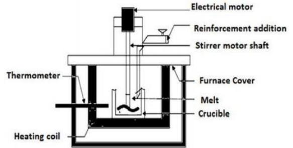
Figure: Stir casting Experimental set up
