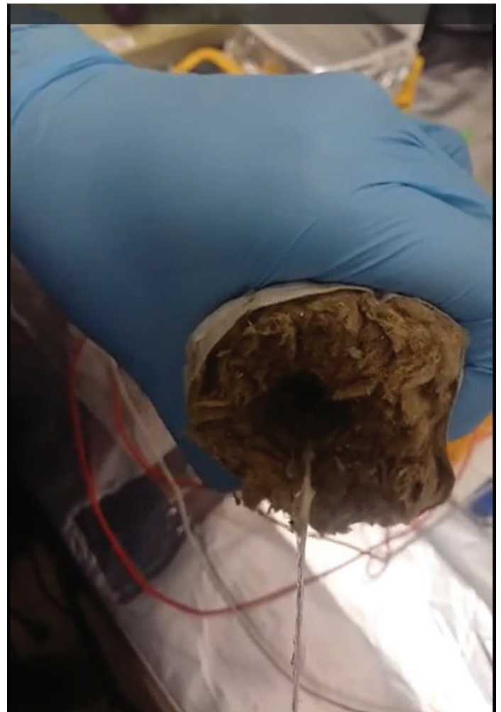
Figure 33 : Melted UHMWPE in Extrusion form
