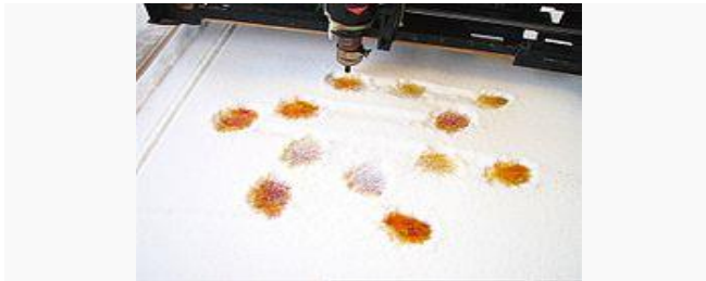
Fig 6. The granular printing system uses heated air and granulated sugar to produce food-grade art objects
