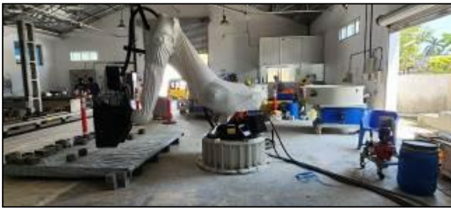
Fig -6: TVASTA’s robotic arm printer at TVASTA Factory at OMR – Chennai. Accelerator dosing pump can be seen on right side.
