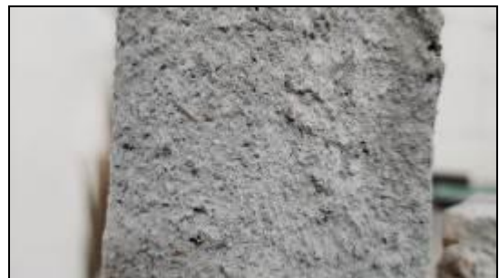
Fig -46: Enlarged section of Trial mix-02 sample: No cold joint, powdery surface texture.
