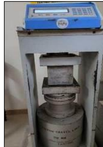
Fig -25: Left – Compression test in progress
