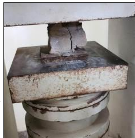
Fig -33: Onsite core samples were tested for compression:
