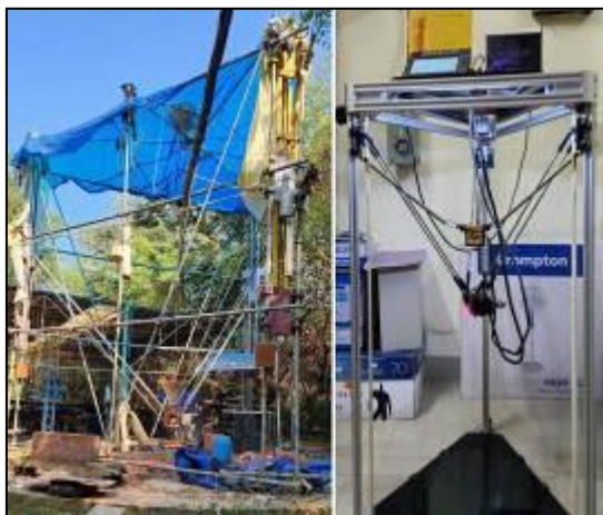
Fig -8: Delta 3D printer at CUSAT, Kochi & Delta 3D concrete printer at Minvayu, Auroville
