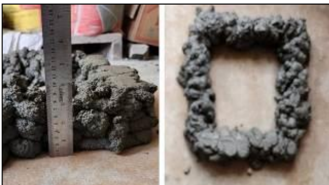
Fig -24: Left – Check for buildability, Right - Hand printed sample
