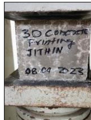
Fig -27: Cube crushed at 28day & Cracking pattern studied
