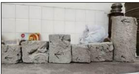
Fig -44: Core samples taken, print direction and top direction marked
