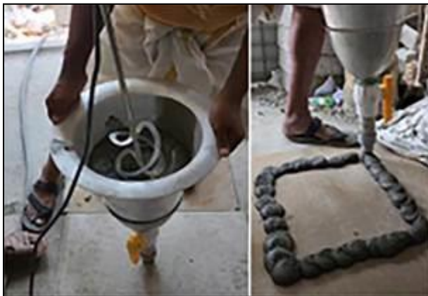
Fig -22: Extrusion by hand printer starts
