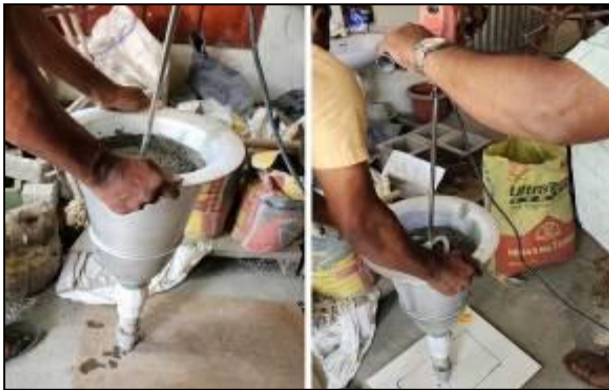
Fig -22: Left - Material mixed in extruder, Right – Extrusion test & check admixture dosage
