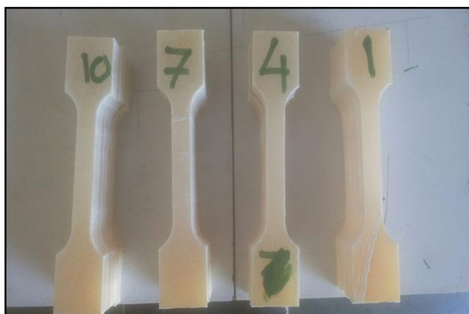
Fig.4. Specimens of the Prepared Formulations According to JANNAF Standard
