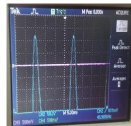
Figure 3: Boosted gain from first to last stage of the output from BPF.
