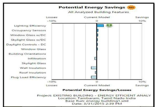
Fig 10 Potential energy savings chart – Optimum model
