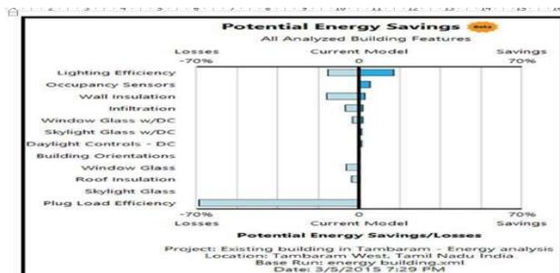
Fig. 9. Alternative trial - Potential energy savings chart
