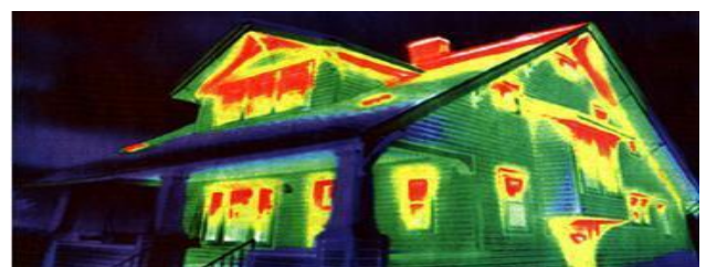
Fig.7. IR testing for leakage in building
