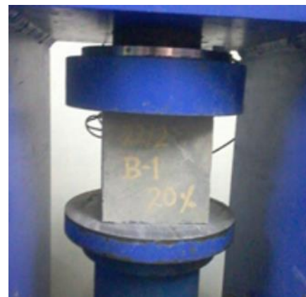
Fig 9 Testing of Specimen in UTM
