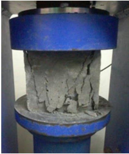
Fig 10 Failure of Specimen
