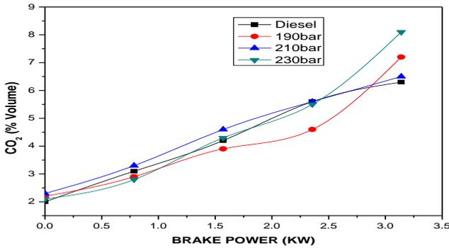
Fig. 3.22: Variation of CO<sub>2</sub> with Brake Power
