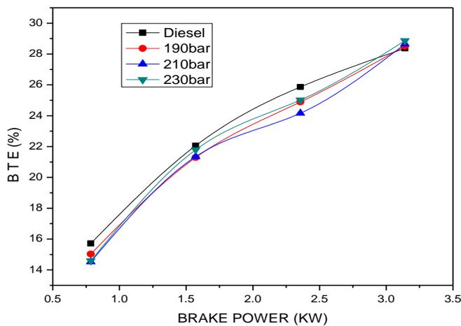
Fig. 3.13: Variation of BTE with Brake Power
