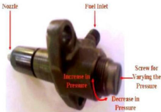
Fig. 2.22: Fuel Injector
