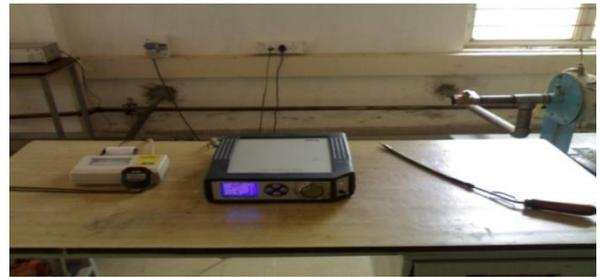
Fig. 2.23: Five Gas Exhaust Analyzer (AVI) with Probe
