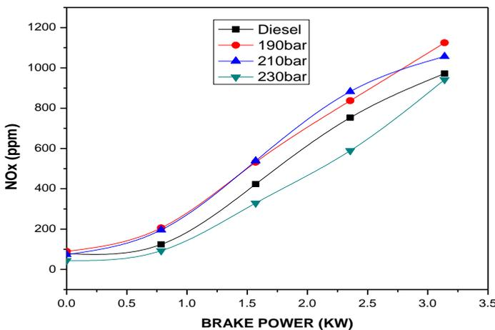
Fig. 3.24: Variation of NO<sub>x</sub> with Brake Power
