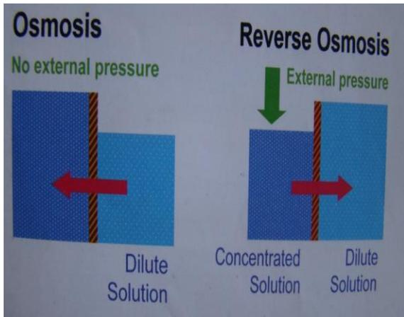
Figure 1 Schematic of Osmosis and Reverse osmosis
