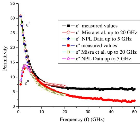
Fig. 2. Variation of dielectric constant ( $\epsilon'$ ) and loss factor ( $\epsilon''$ ) of methanol with frequency at room temperature ( $25^{\circ}\text{C}$ )
