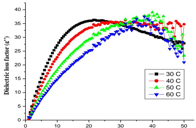
Fig. 4. Frequency dependence of the dielectric loss factor ( $\epsilon''$ ) of water at indicated temperatures
