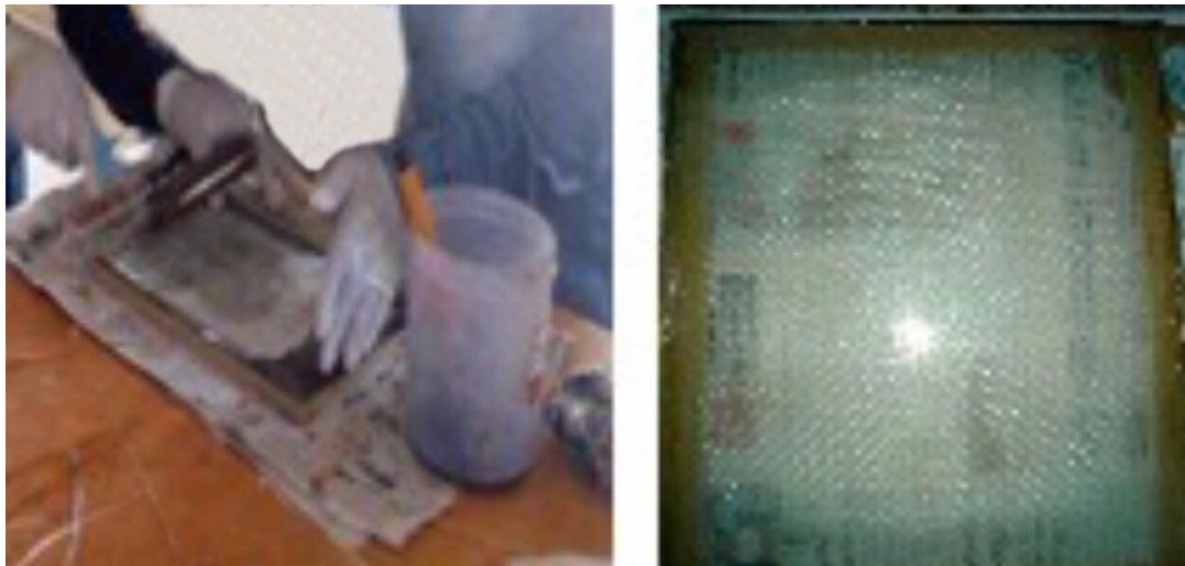
Fig.4.4 Pasting the second layer of Epoxy and curing the sample at room temperature
