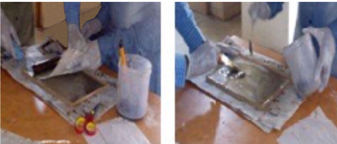
Fig.4.3 Pasting the first layer of Glass fibre and applying the second layer of Epoxy
