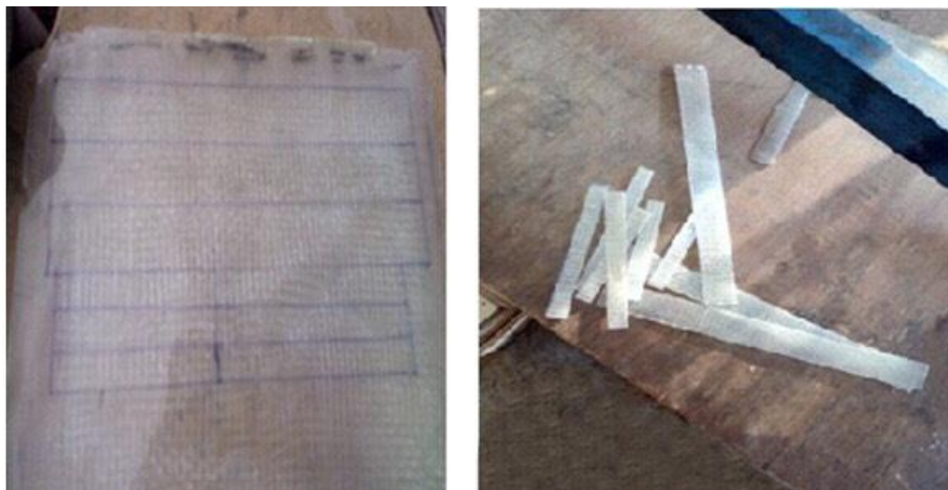
Fig.4.6 Marked glass epoxy composite and ASTM/ISO based standard specimens
