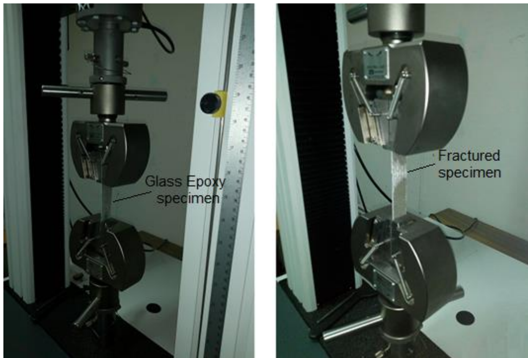
Fig.4.9 Glass epoxy specimen before and after failure during tensile test
