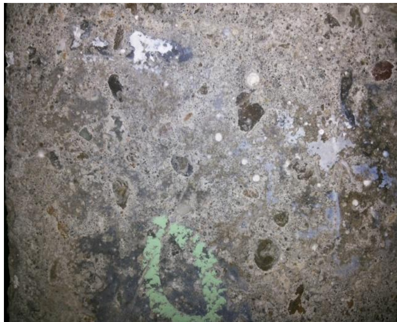
Fig. 3.10: Control concrete specimens after 365 days period of immersion in 10% magnesium sulfate solution (Concrete 'X')
