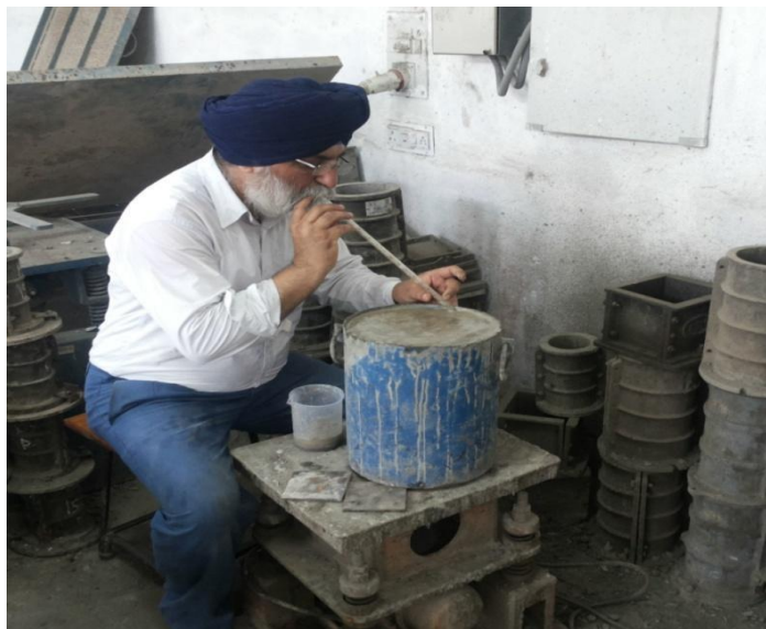
Fig. 3.4: Experimental set up for collection of bleeding water from the surface of concrete
