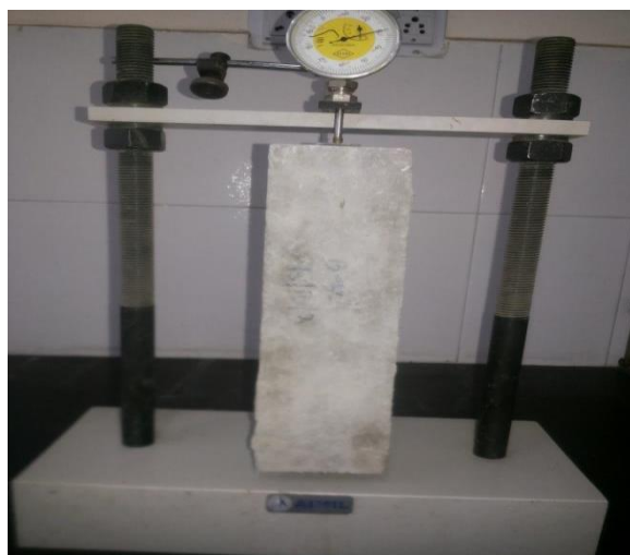
Fig. 3.9: Experimental set up for measuring length change
