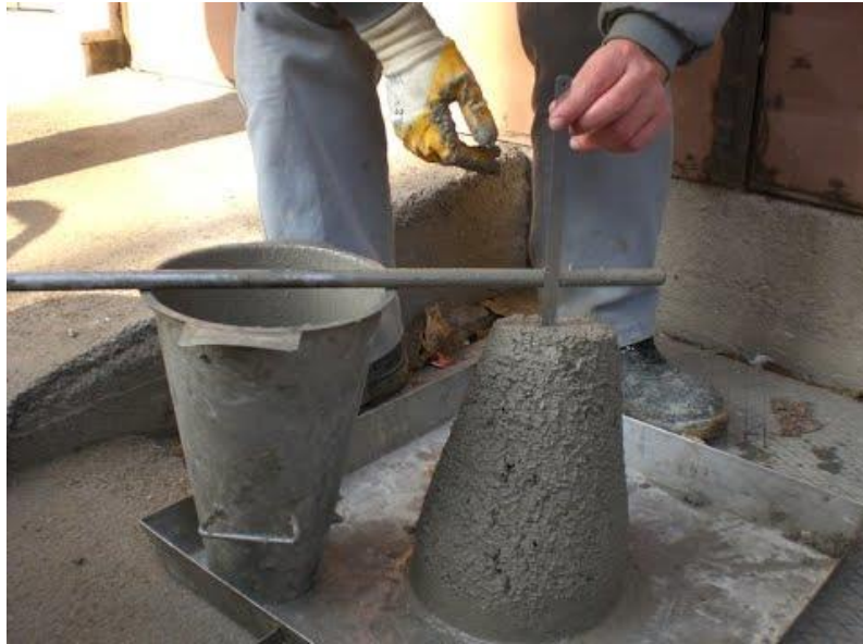
Fig. 3.2: Experimental set up for measuring slump of fresh concrete
