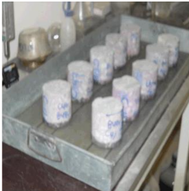
Fig. 3.5: Experimental set up for measuring sorptivity of concrete
