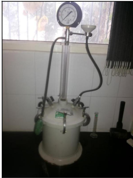
Fig 3.3: Experimental set up for measuring air content in fresh concrete
