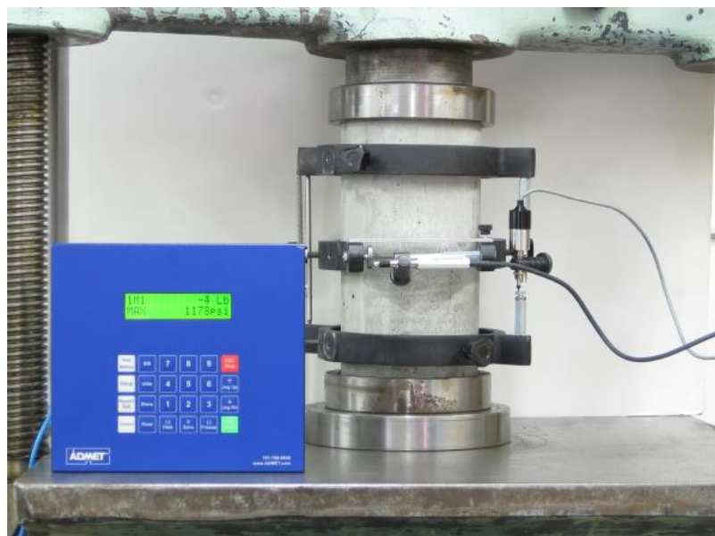
Fig. 3.8: Experimental set up for measuring modulus of elasticity of concrete
