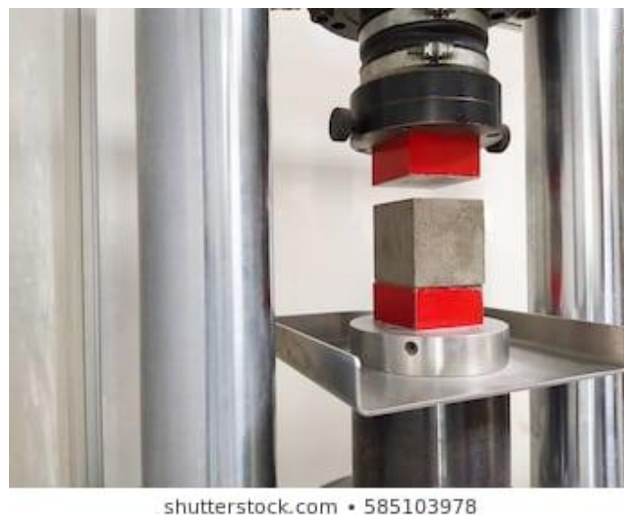
Fig. 3.6: Compression testing machine (Capacity 3000 kN)
