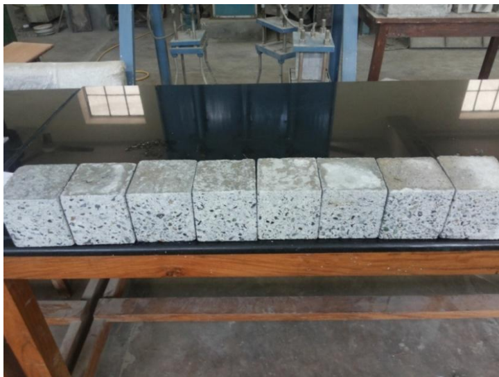
Fig. 3.12: Deterioration of specimens after 84 days of immersion in 3% sulphuric acid solution
