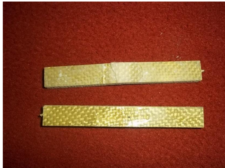
Figure 4.5 Photographic view of GFRP-polyester after flexural fracture
