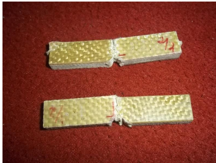
Figure 4.8 Photographic view of GFRP-epoxy after impact fracture
