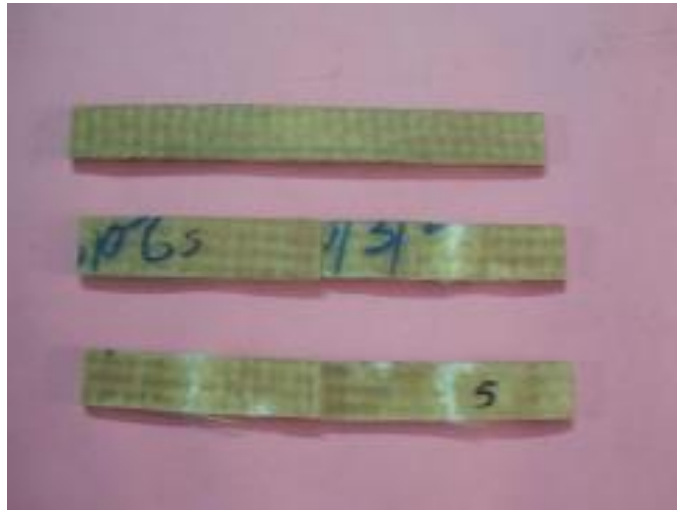
Figure 4.4 Photographic view of GFRP-polyester after flexural fracture
