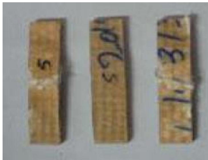
Figure 4.7 Photographic view of GFRP-epoxy after impact fracture
