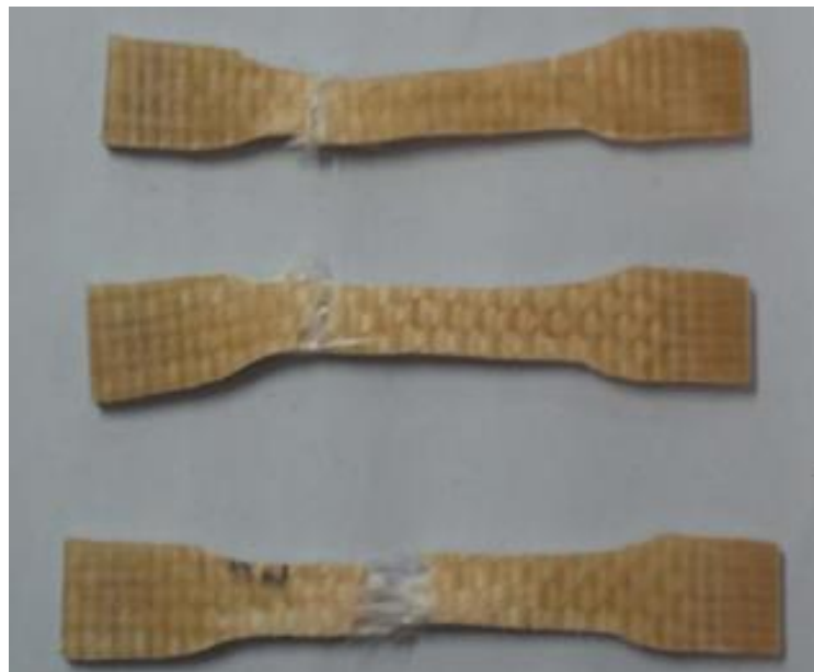
Figure 4.1 Photographic view of GFRP-polyester after tensile test
