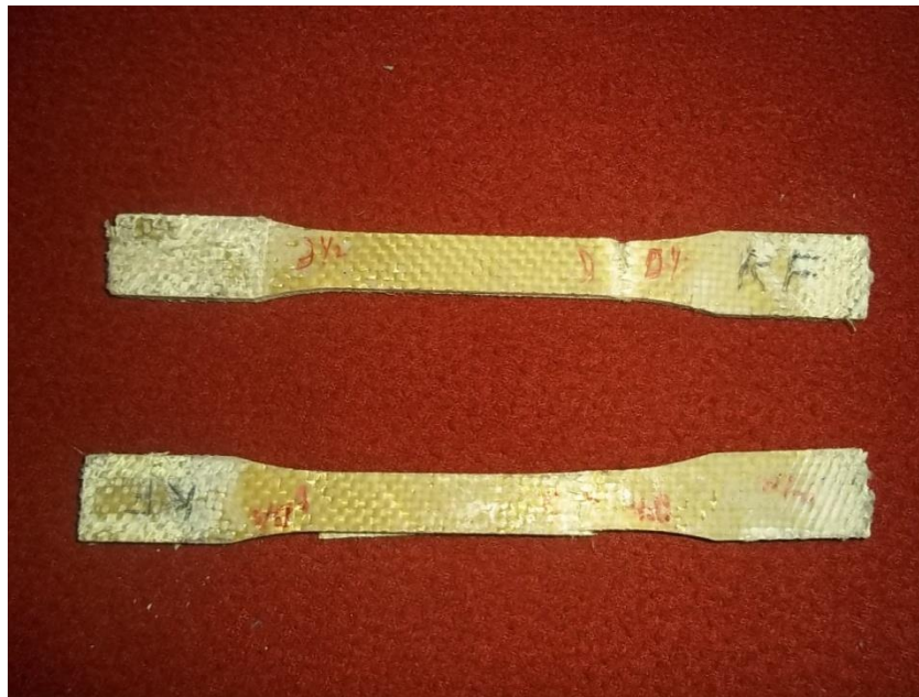
Figure 4.2 Photographic view of GFRP-epoxy after tensile test
