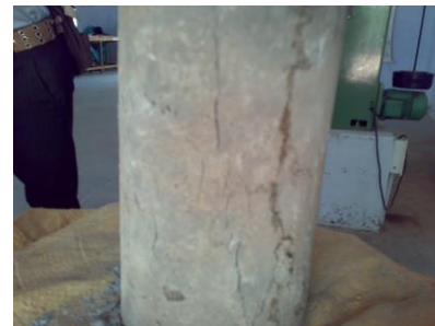
Fig.3. Crack analysis on cylinder
