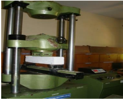
Fig.3. loading diagram for flexure strength
