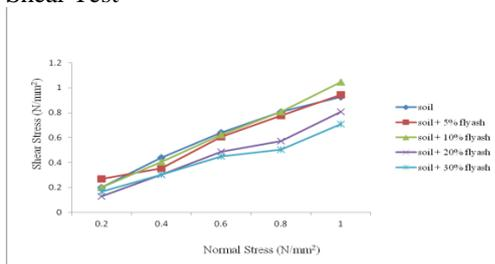
Figure 5. Comparison of shear strength of soil with various proportion of fly ash
