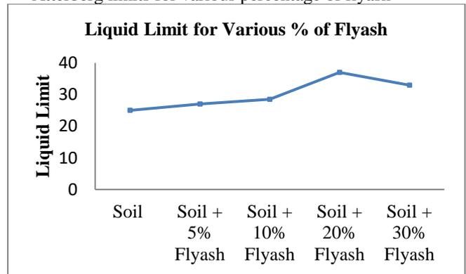
Figure 2. Liquid Limit for Various % of Flyash
