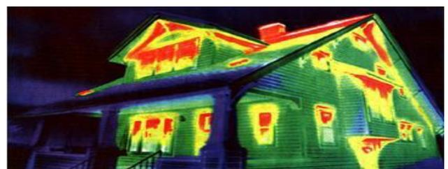
Fig.7. IR testing for leakage in building
