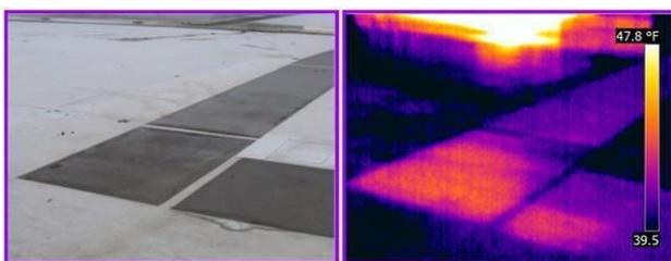
Fig.5. IR Imaging of roof leak
