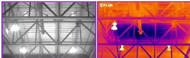
Fig.4. IR Imaging of Roof Truss
