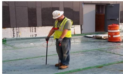
Fig.2. EFVM testing for leakage in roof
