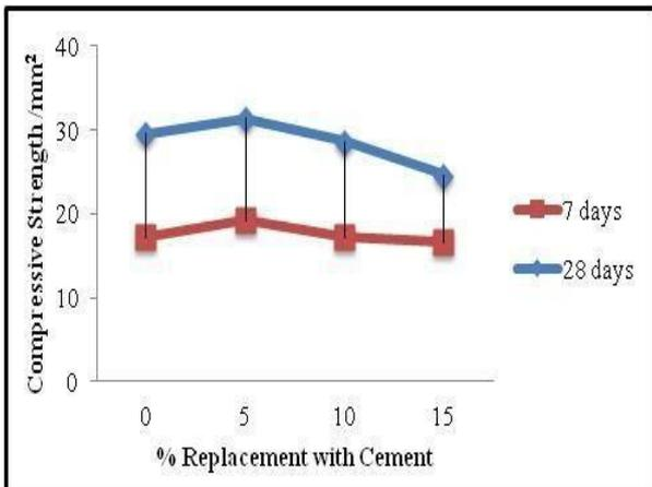
Fig. 1. Compressive Strength at 7 and 28 days
