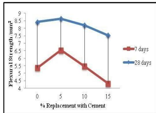
Fig. 3. Flexural Strength at 7 and 28 days
