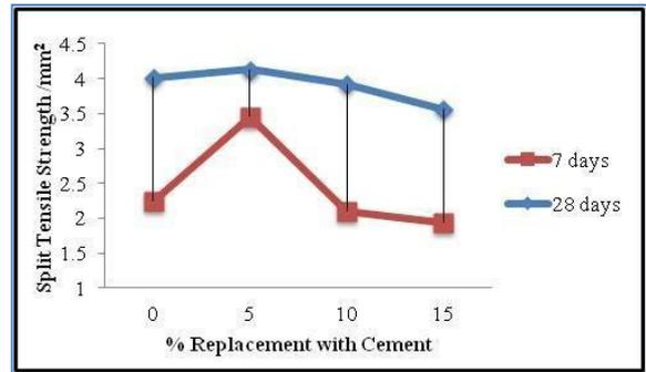
Figure 2. Split Tensile Strength at 7 and 28 days
