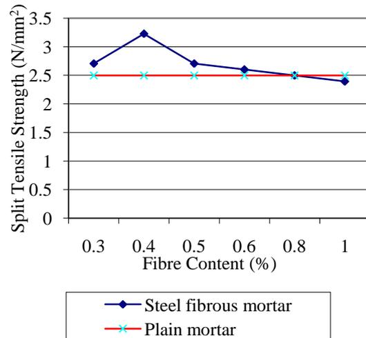
“Fig. 7 Split Tensile strength with various fibre dosages for 28 days curing”
