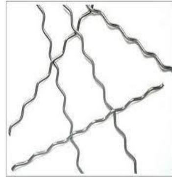
“Fig. 1 Physical appearance of short steel fibres”
