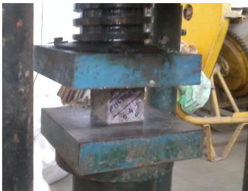
**“Fig. 2(a) Compression test”**
