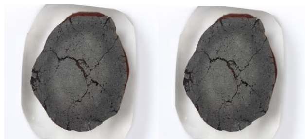
Figure 3 Picture of the cut etched sample reduced in 5 l/min H 2 for CVRD pellets
