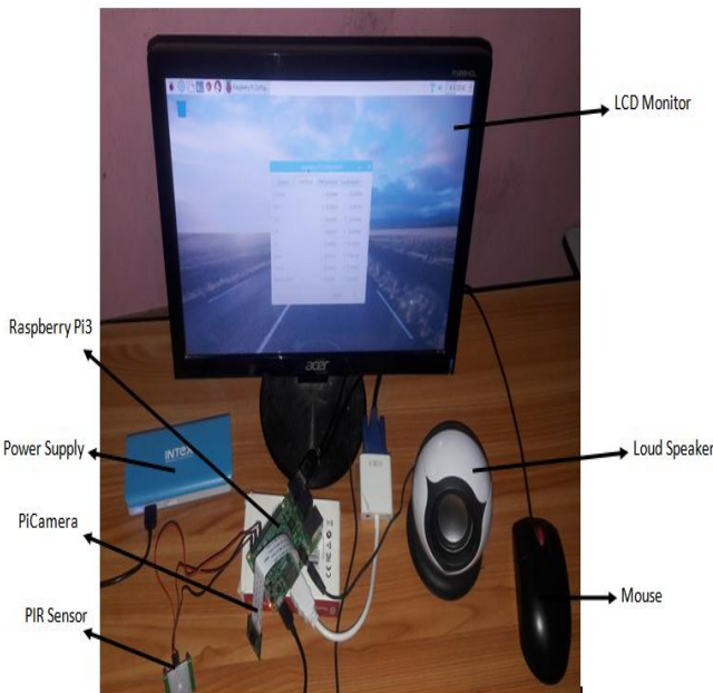
Figure 5: Working Experimental setup for ECU
