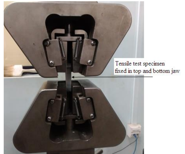
Fig.4 During tensile testing of composite material
