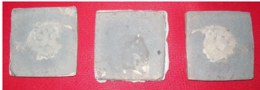
Fig. 7 Debonding of AZ91 with SiC reinforced plates
