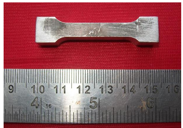
Fig.5. Tensile specimen of composite material
