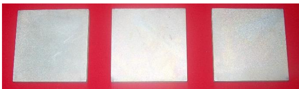
Fig. 1 AZ91 Magnesium plates before diffusion bonding
