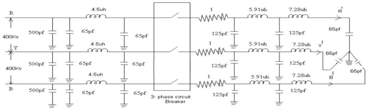
Fig. 1 Equivalent circuit for 10mtrs. Length in a 3 -phase to 2-phase 400kv GIS
