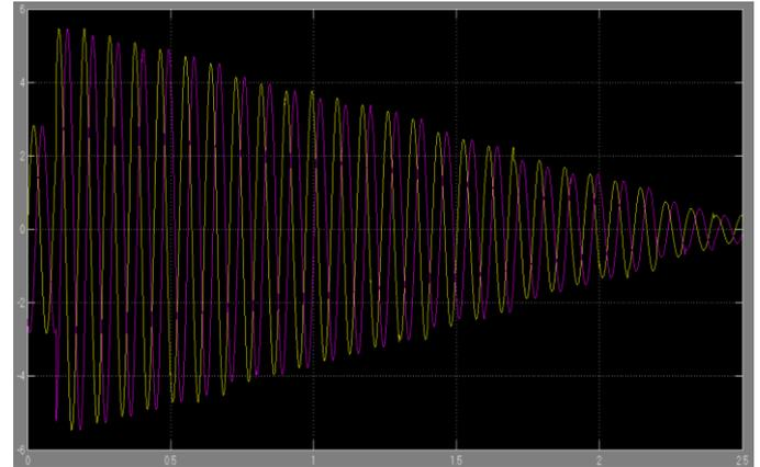
Fig.8 Transient voltage waveform during second re-strikes for 10mts length in a 2-phase 400kv GIS
