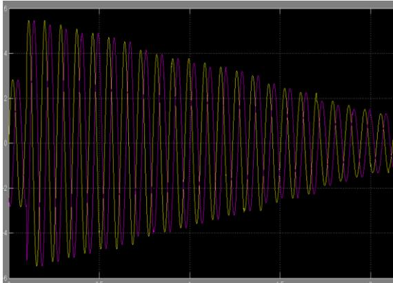
Fig 6 Transient voltage wave from during closing operation of CB for 10mts length in a 2-phase 400kv GIS
