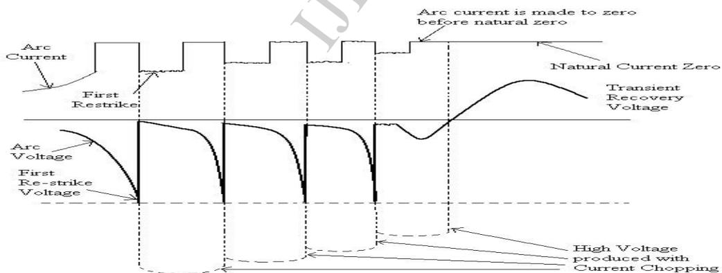
Fig 3 waveform of over voltage with current chopping
