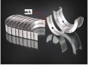
Fig 2: Nick on Bearing Halve.
